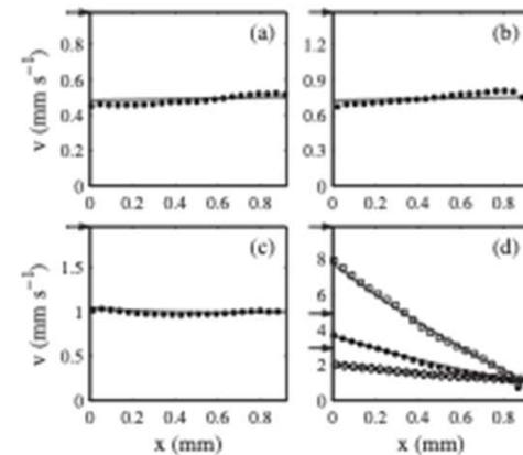
FIG. 3. Velocity profiles in the nonadhesive emulsion for (a)  $v_0 = 0.98$ , (b)  $v_0 = 1.47$ , (c)  $v_0 = 1.96$ , and (d)  $v_0 = 2.94$  (○), 4.90 (●), and 9.79 mm s<sup>-1</sup> (□). Arrows indicate the wall velocity  $v_0$ . The solid lines correspond to solid body rotation in (a) and (b) and to the Herschel-Bulkley model with  $\sigma_0 = 58.0$  Pa,  $A = 11.4$ , and  $n = 0.45$  in (c) and (d) [see Eq. (3)].
