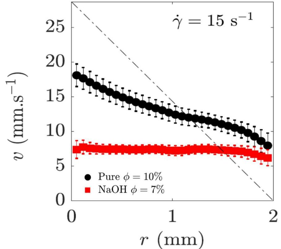
Pure calcite paste never shows shear-band
