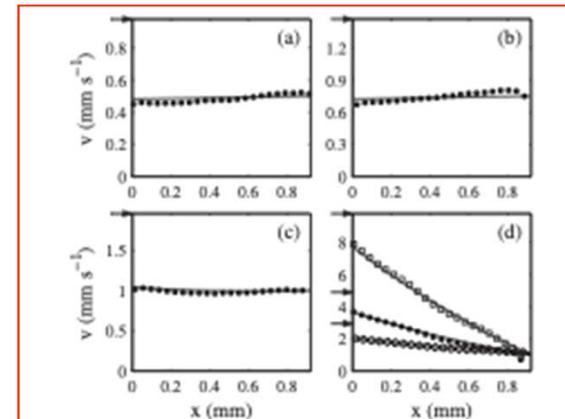
FIG. 3. Velocity profiles in the nonadhesive emulsion for (a)  $v_0 = 0.98$ , (b)  $v_0 = 1.47$ , (c)  $v_0 = 1.96$ , and (d)  $v_0 = 2.94$  ( $\circ$ ),  $4.90$  ( $\bullet$ ), and  $9.79$   $\text{mm s}^{-1}$  ( $\square$ ). Arrows indicate the wall velocity  $v_0$ . The solid lines correspond to solid body rotation in (a) and (b) and to the Herschel-Bulkley model with  $\sigma_0 = 58.0$  Pa,  $A = 11.4$ , and  $n = 0.45$  in (c) and (d) [see Eq. (3)].
