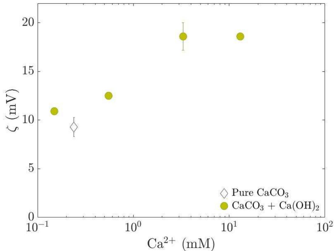
Adsorption of  $\text{Ca}^{2+}$  at calcite surface
